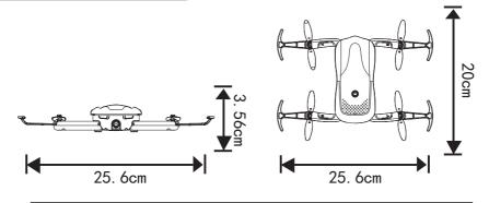
Drone length: 20cm Drone width: 25.6cm Drone height: 3.56cm Motor size:  $\phi$ 8x16
